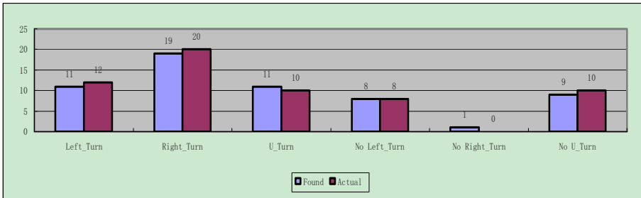
Fig. 2. Mining result of trajectory near road intersection (the blue column is figure of mining result, the violet one is figure of filed survey)
